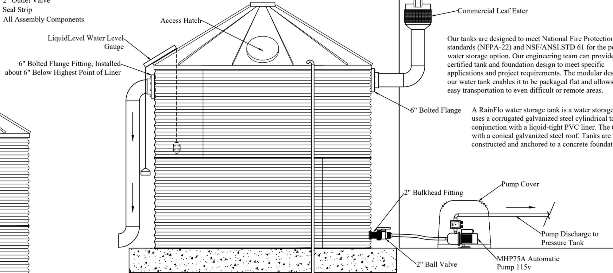
Our tanks are designed to meet National Fire Protection standards (NFPA-22) and NSF/ANSI.STD 61 for the potable water storage option. Our engineering team can provide certified tank and foundation design to meet specific applications and project requirements. The modular design of our water tank enables it to be packaged flat and allows for easy transportation to even difficult or remote areas.
